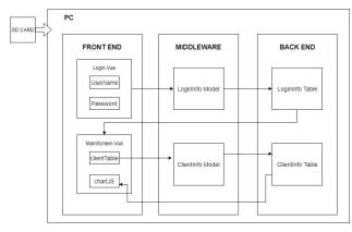
Figure 19 - Block Diagram of the Software [32]
